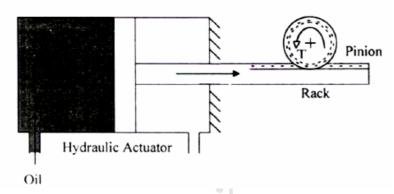
76. If the diameter of the piston is 0.05 m, the force (kN) generated on the piston is
